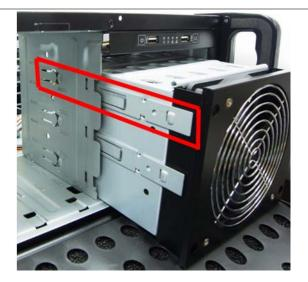
4. In order to insert the cage into the ODD tray, you will need to rotate the cage so the cage rail will match with the side.
