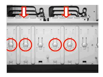
1. First press the two round shape button using your thumbs, then use your index finger to push the 3.5" module to remove it.
