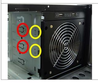
**6.** You will see that the Cage Rails fit right into the ODD tray's hole in the yellow circles.
