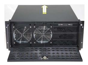
2. Once the screws removed, push the top cover to remove from the chassis.
