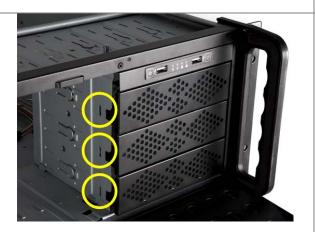
**3.** Using a flathead screw driver to press the Yellow circle to move the front panel out.
