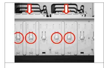
1. First press the two round shape button using your thumbs, then use your index finger to push the middle 3.5" module to remove it.
