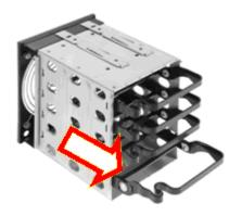
**3.** Pull the HDD tray out from the module to begin installation.
